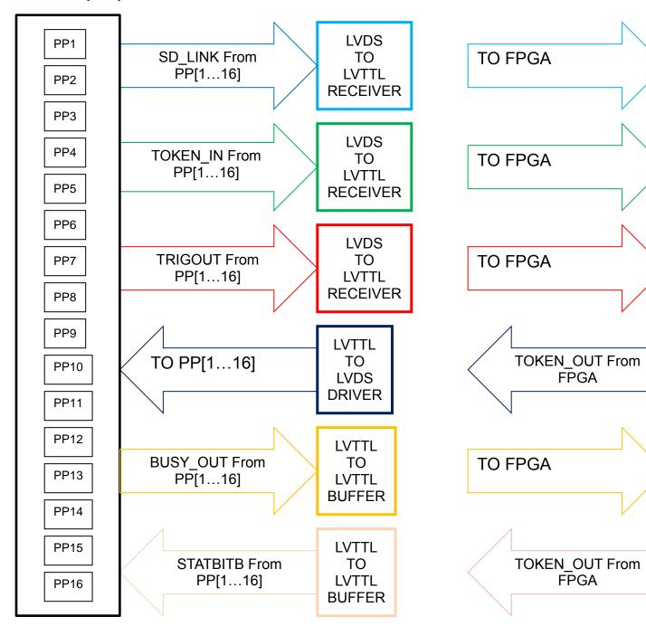
Figure 5: Shows the LVDS to LVTTL signal connections from the Payload Modules to the FPGA
