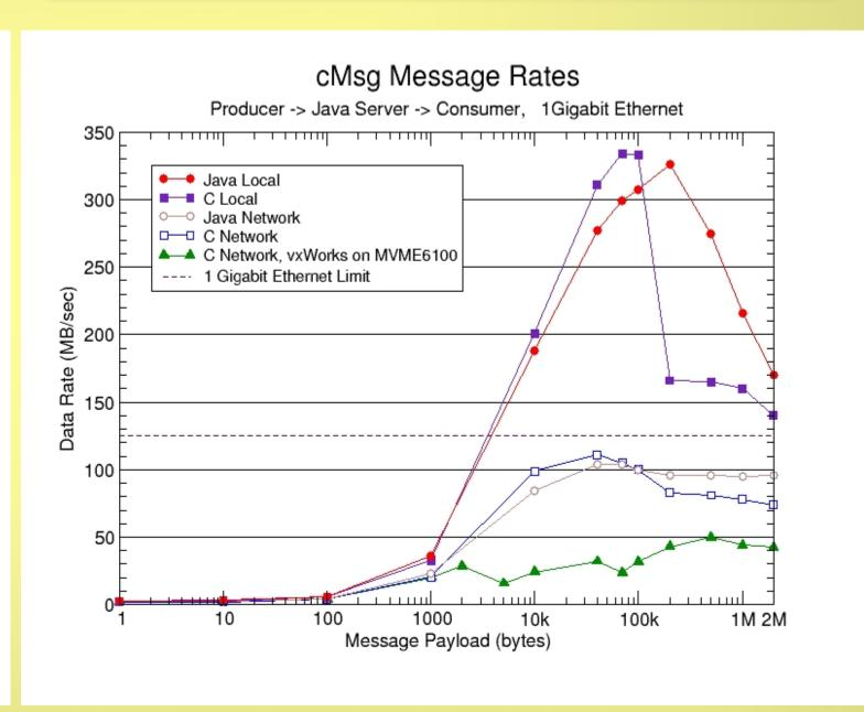
cMsg server running on a 2.4 GHZ quad-Opteron, RHEL3, Gbit Ethernet, Cisco Catalyst 4000 switch
