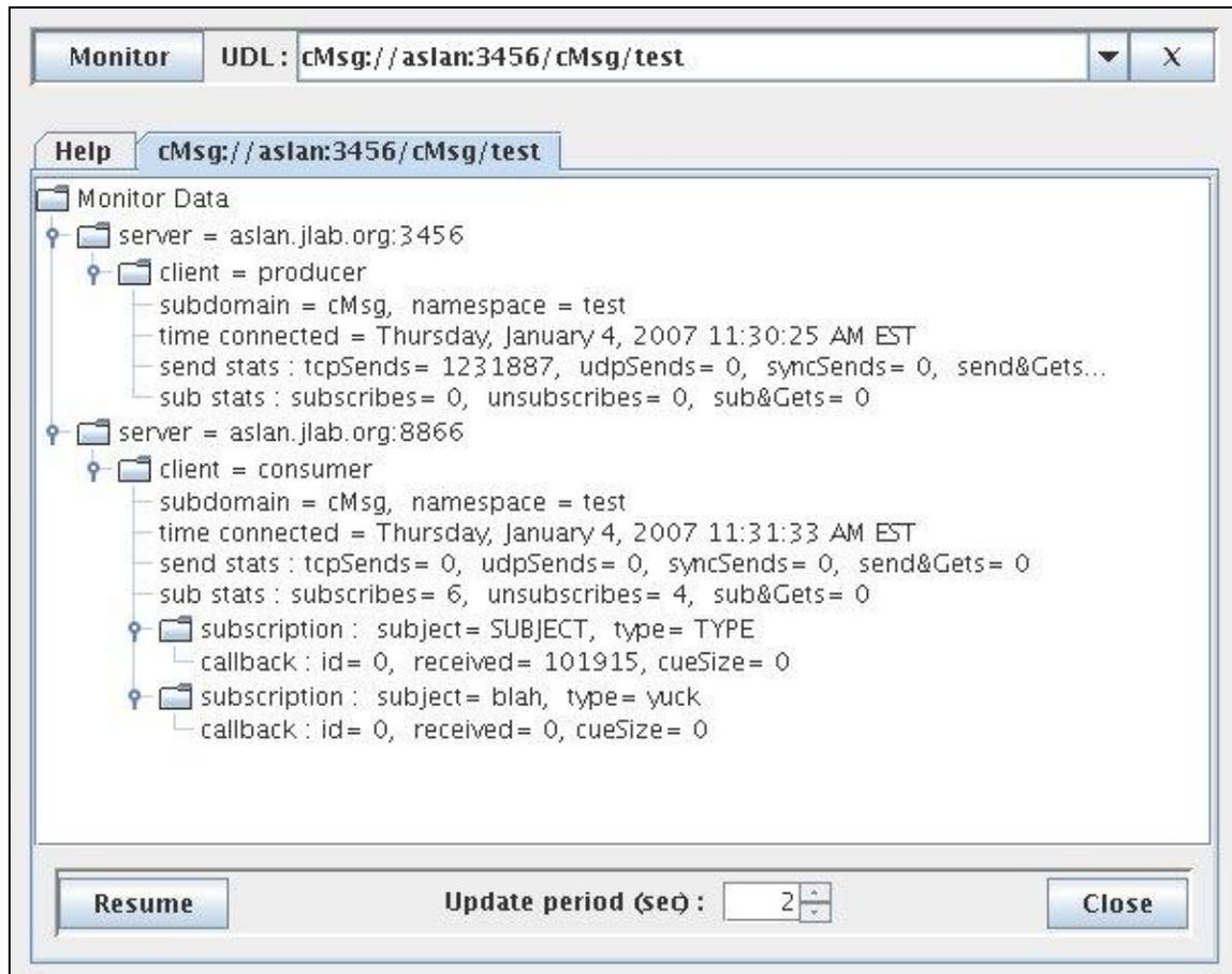
It's fairly self-explanatory. Just type in the UDL, hit "Monitor", and a new tab will be added with all the monitoring information about the cMsg cloud of servers and all their clients. The monitoring can be paused/resumed, closed, and the update period can be changed.
