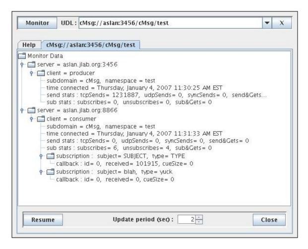
It's fairly self-explanatory. Just type in the UDL, hit "Monitor", and a new tab will be added with all the monitoring information about the cMsg cloud of servers and all their clients. The monitoring can be paused/resumed, closed, and the update period can be changed.
