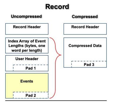
Each record has a header. The header is followed by an index of events lengths – one word per length in the unit of bytes. This index is **not** optional.
