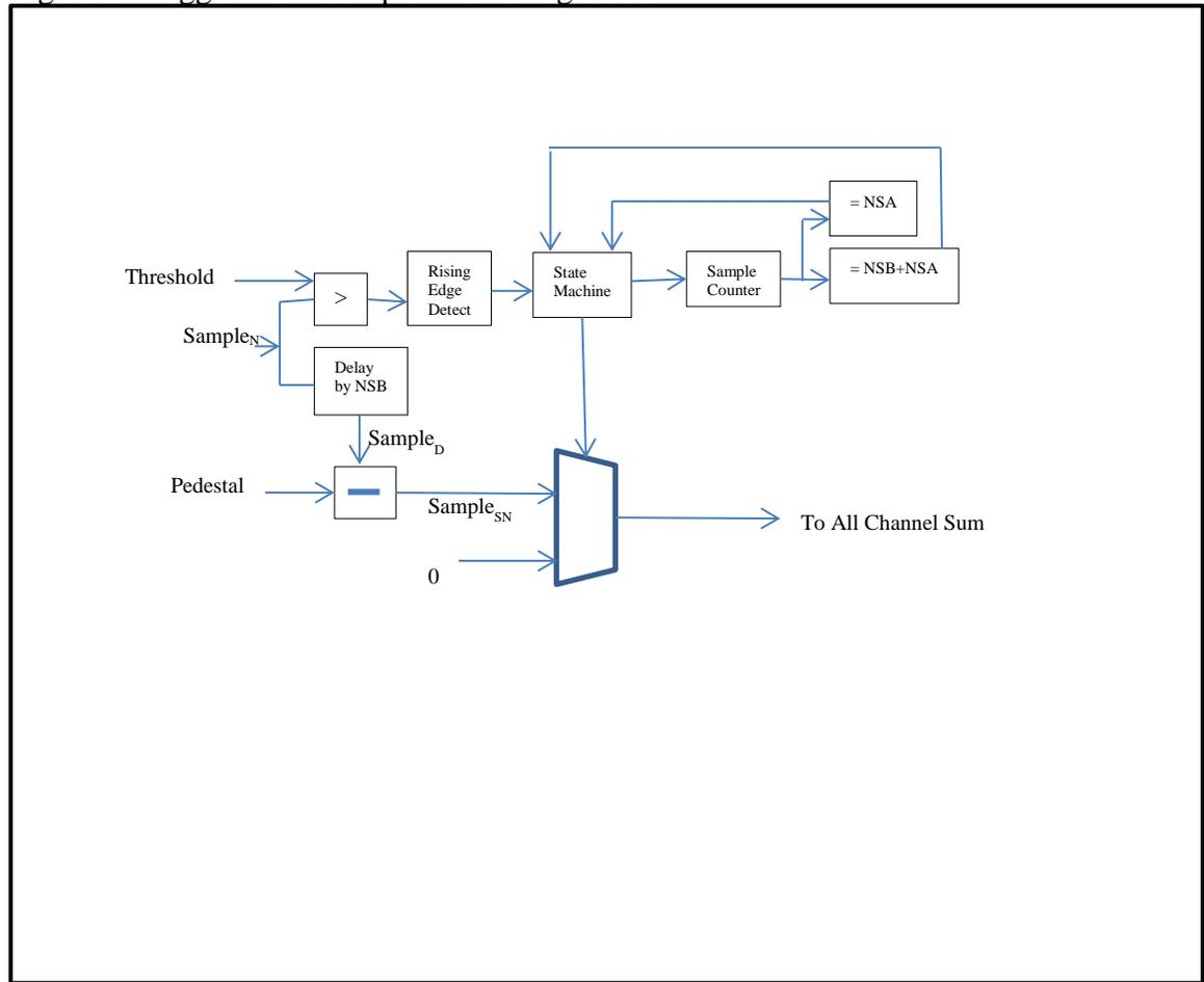
Figure 4. Example for Trigger Path Sample Processing Code:
