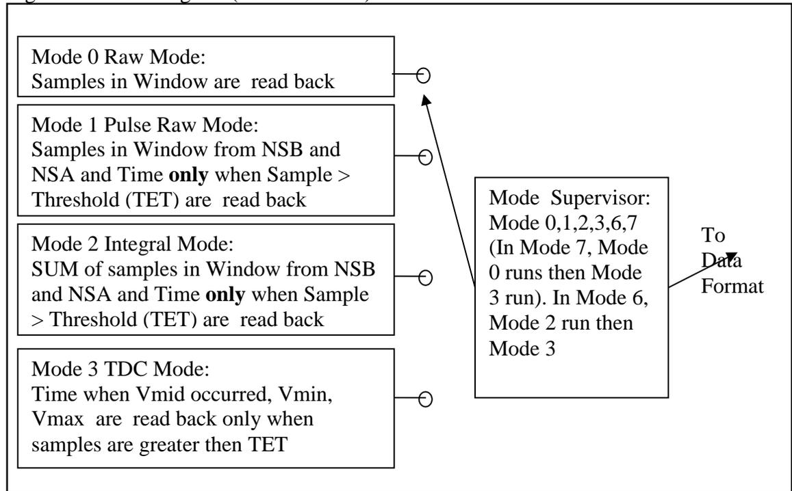
Figure 3. Trigger Path: Sample Processing Code
