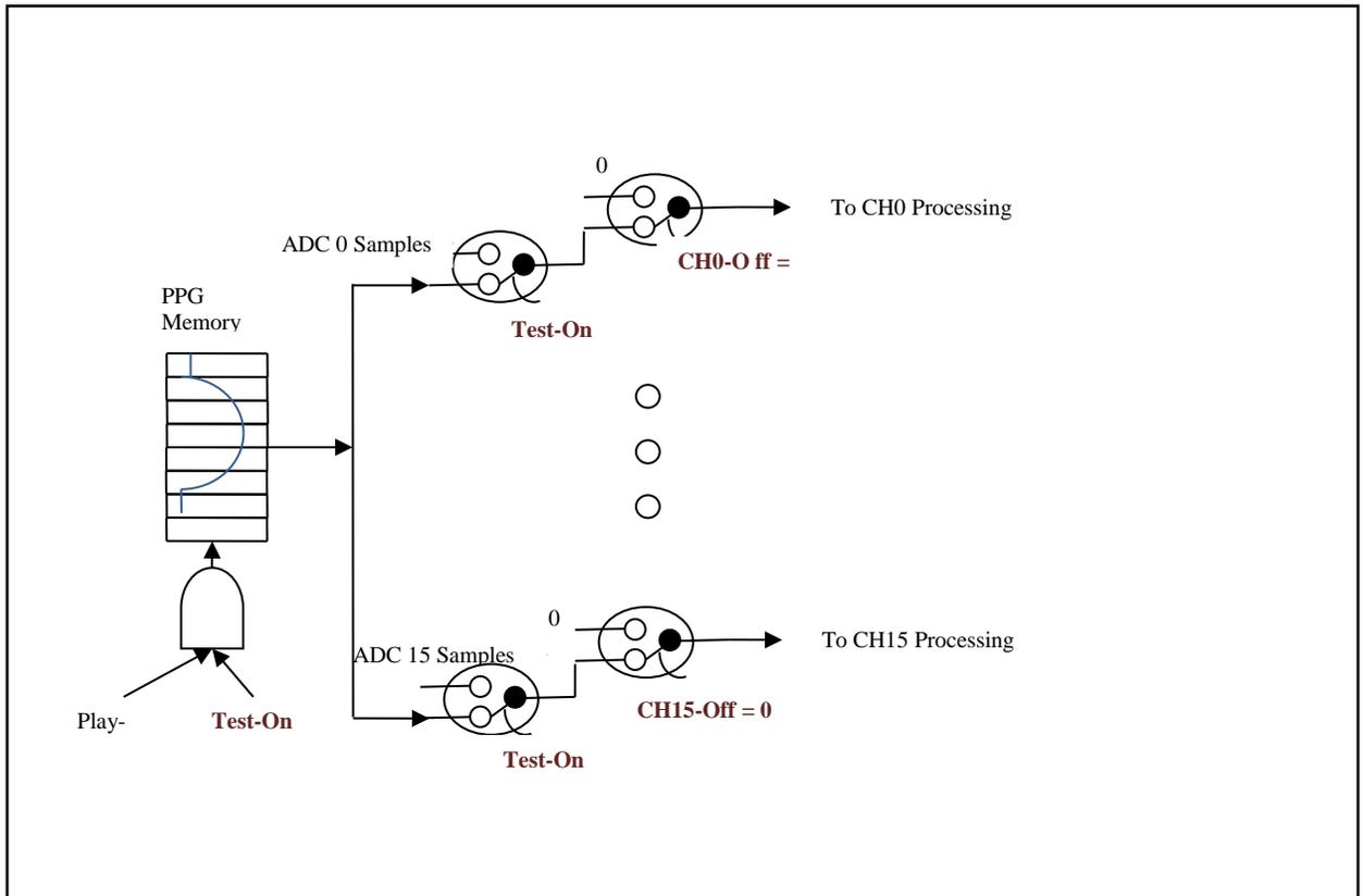
Test On is bit 6 of Configuration register. CHx-Off are bits 8-15 of configuration register.
