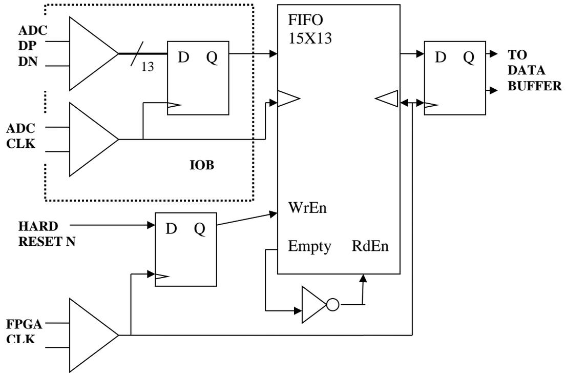
Each ADC has 12 bits data, an overflow, and an ADCCLK. The ADC Input Resync captures ADC's data and overflow bits with ADC's output clock to a 15 deep (smallest allow by ISE) by 13 bits FIFO. The FIFO allows the FPGA main CLK to be independent of ADC clock. The FPGA main CLK clocks the data out of FIFO and send to the Data Buffer Block.
