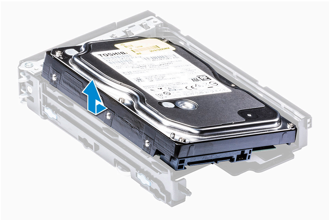
b Lift the hard drive out of the bracket.
