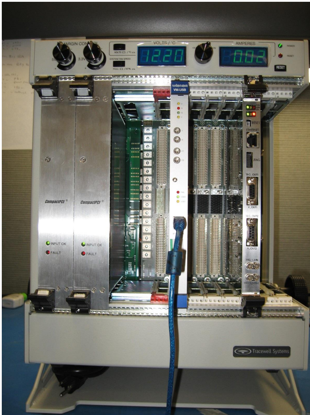
Figure 6. Weiner VME USB and Fast Light Pulser Board Setup for FastLightPulser.exe Demo GUI Program
