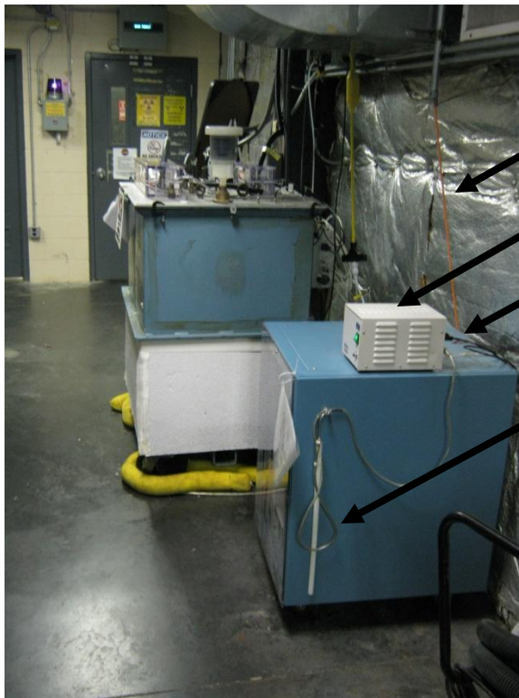
Figure 3: Rack that houses the Helicity Control Board. This crate is powered by an Isolation Transformer and is floating at 65 VAC. Please follow safety procedure when working in this rack. The ground pin of the Isolation Transformer power cable is removed.
