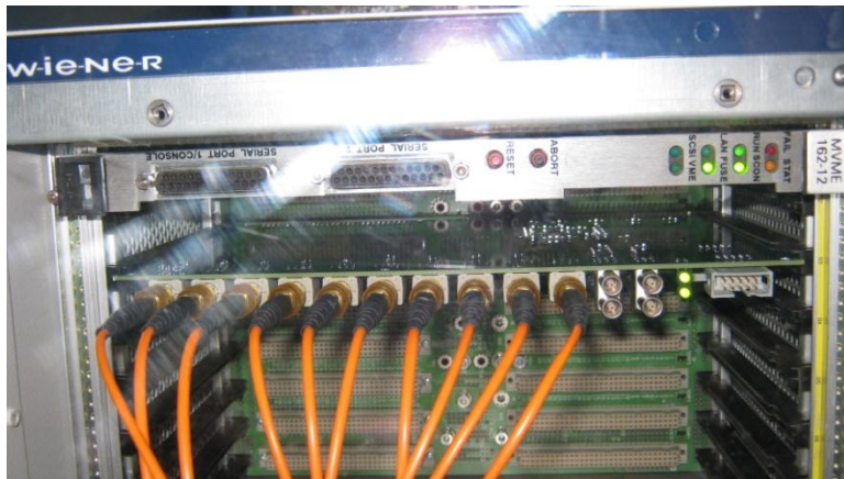
Figure 4: Helicity Control Board and its Crate. This is IOC "iochelgen". (Remove the two un-used modules in this crate. Add a front panel to the Board).
