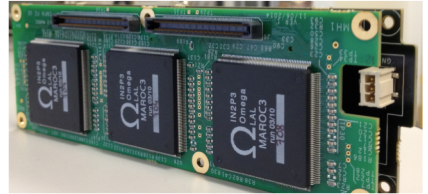
ASIC board produced for the RICH detector for CLAS12 with MAROC chips installed
