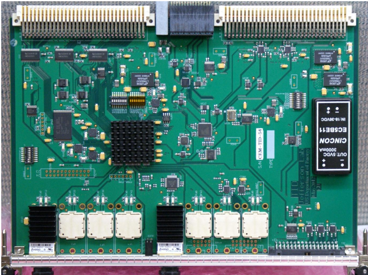
Figure 7 Trigger Interface card. The TI shares the same PCB design as TD, but the components are populated differently from the TD.
